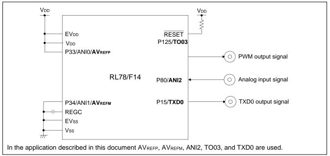
Figure 2.1 Connection Diagram of Pins Used
