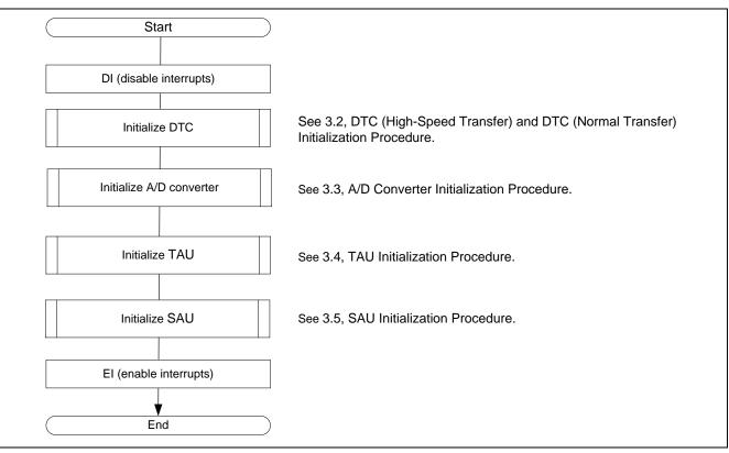
Figure 3.1 Peripheral Function Initialization Procedure
