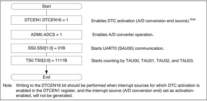
Figure 3.9 Procedure for Enabling Peripheral Functions (DTC (High-Speed Transfer) Transfer Start)
