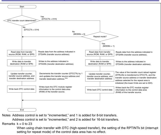
Figure 1.5 Flowchart of DTC (Normal Transfer) Internal Operation
